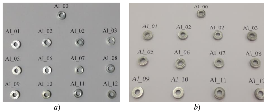
Fig. 3. a) rings before pressing; b) rings after pressing
